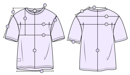
Figure 6: T-shirt - Points of Measurement
