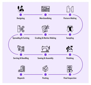
Figure 3: T-shirt Manufacturing Process
